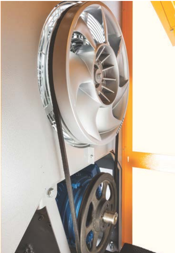
Interior view of PE-VE: Adjustment of the V-belt is not necessary because of the vertical format and suspended motor mounting.
