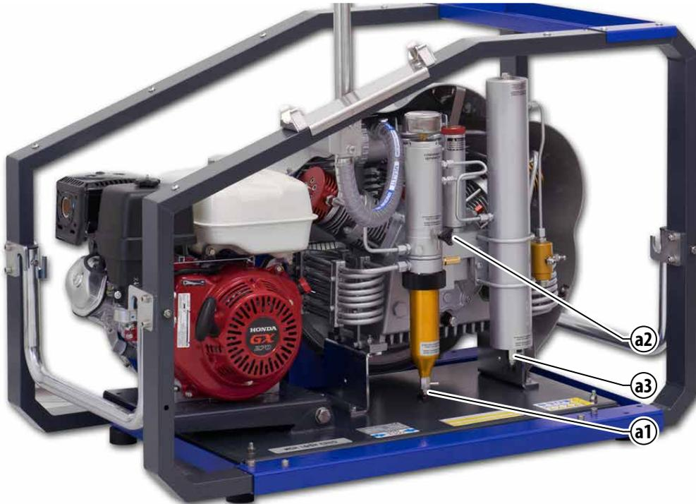
If the condensate needs to be drained manually, use the drain taps (a) and collect the condensate in a suitable container. Re-close the taps. An outflow of condensate water with lubricating oil is normal during refills: the quantity will depend on the level of humidity in the air.
